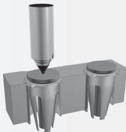
Automatic mounting by a chip mounter
