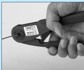
①Insert the terminal into the crimping tool. Insert the wire into the hole of the terminal.
