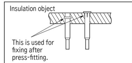
\* The main body (VP) is inserted into the dimension of D + E (①), E (②, ③).
