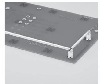
As the upper part of the insulation type can turn, please turn the lower part after soldering and align.
