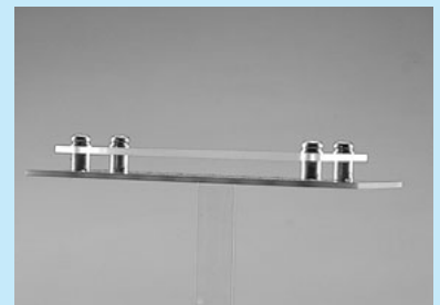
Condition of fitting the panel to the printed board
